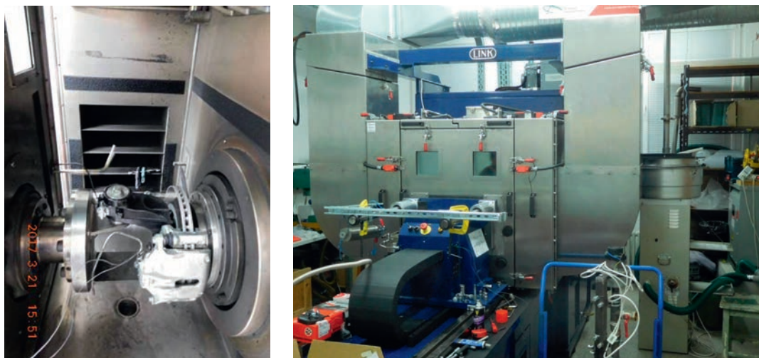
Fig. 1. Brake assembly (left) and brake dynamometer enclosure (right).
